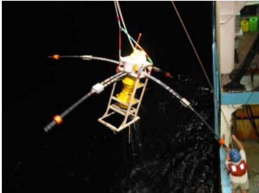
Photo 7. OBEM (TT1); site 8) pulled out of water.
