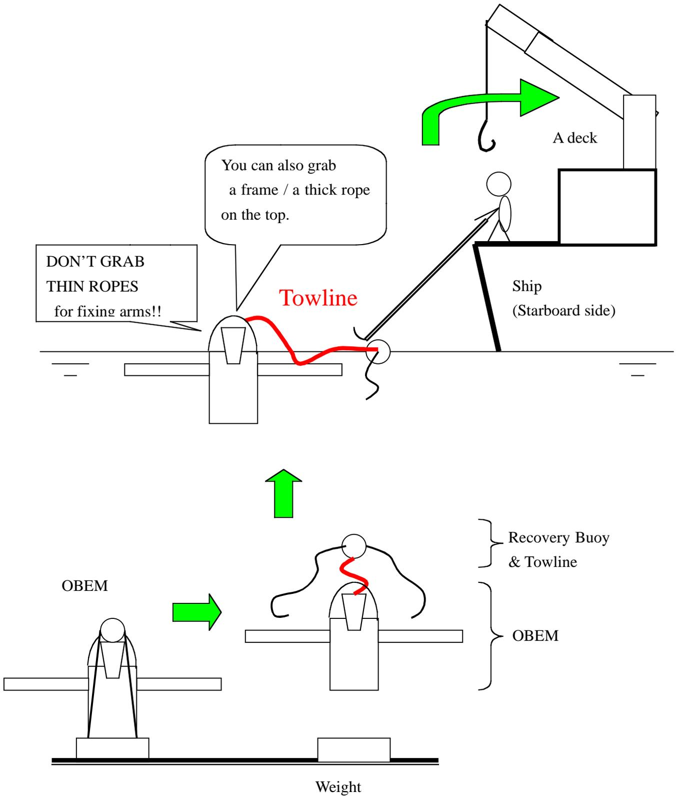
**Fig. 6. How to release the towline for the OBEM**
