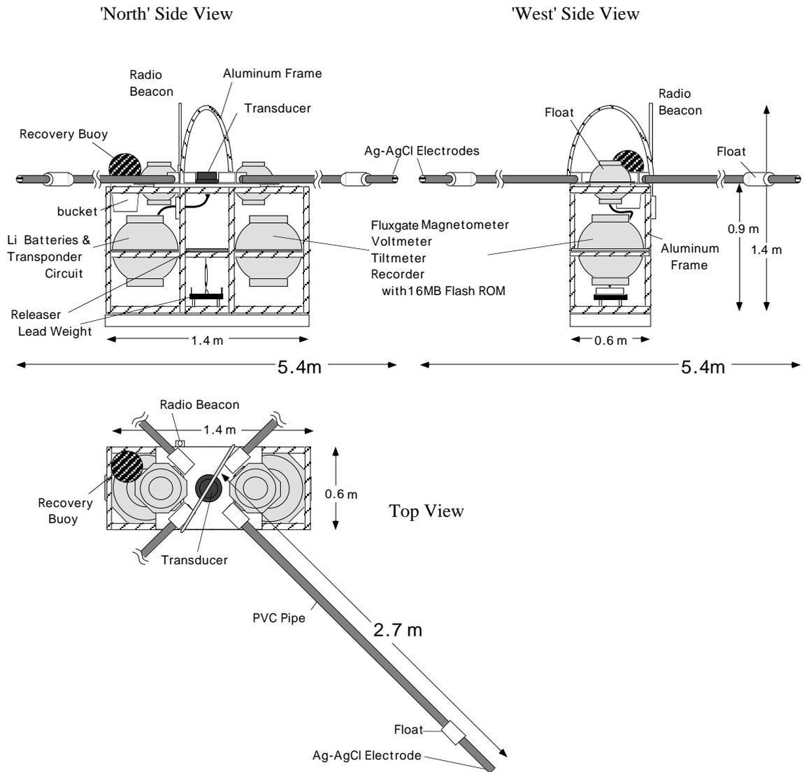
Fig. 2. Side and top views of Japanese OBEM (half type). This OBEM is deployed at site 9 in the Mariana region (see maps shown later). This was newly developed in 1999. Its total weight in air is 130kg (without the lead weight).
