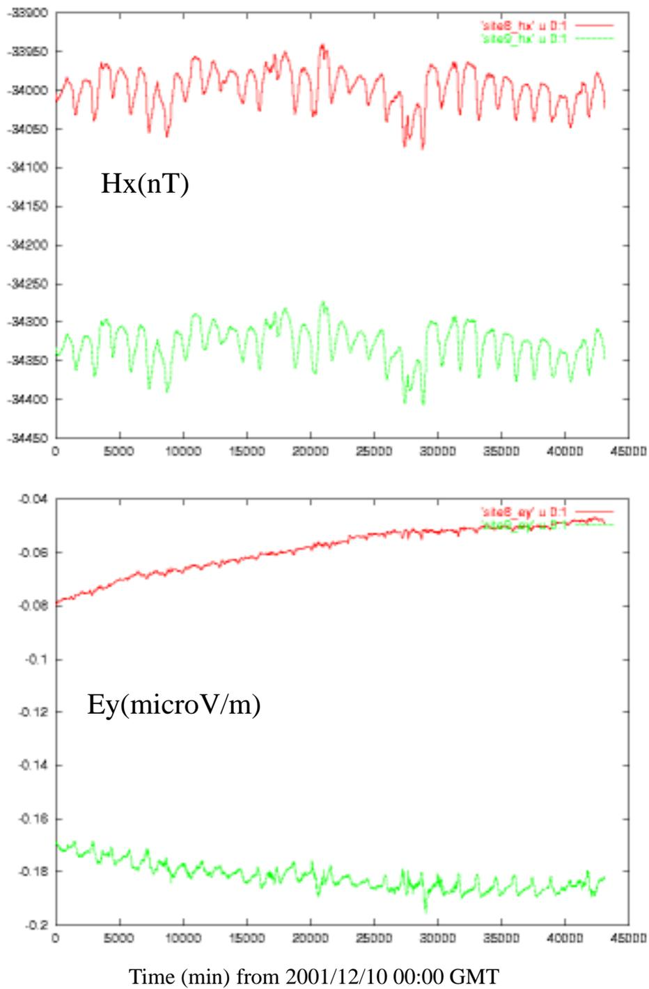
Fig 7. An example of observed magnetic and electric fields at sites 8 (red) and 9 (green). X and Y axes for observation turn to south and east approximately. The time series is plotted from 2001/12/10 00:00:00GMT to 2002/01/08 23:59:00 (30 days). 1 data point = 1 minute.
