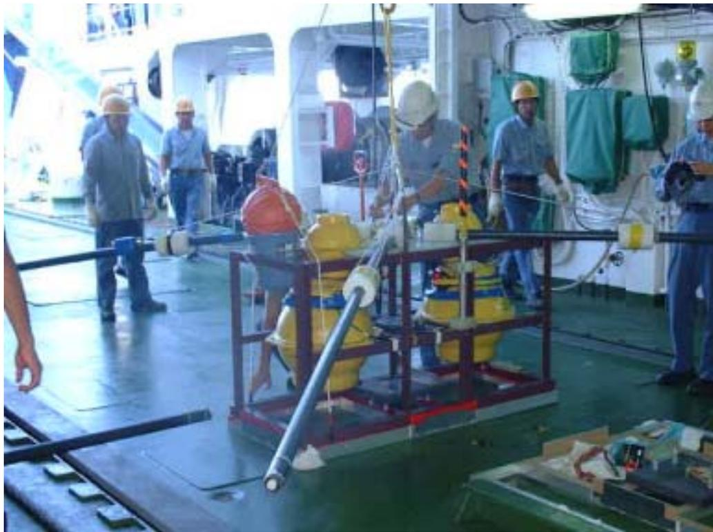
Photo 4. OBEM Half Type built in hanger deck.
