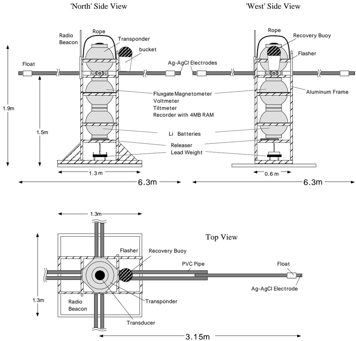
Fig. 1. Side and top views of Japanese OBEM (tall type). These OBEMs are deployed at site 8 and 10 in the Mariana Region (see maps shown later). This tall type has been used for these 10 years. Its total weight in air is 130kg (without the lead weight).
