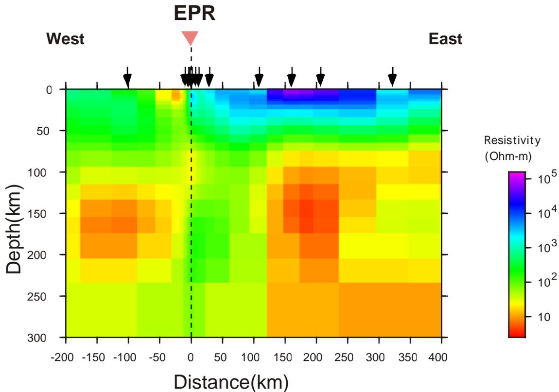
Fig. 3. Resistivity structure below the East Pacific Rise. Arrows indicate OBEM locations. Red color indicates ‘low resistive’ or ‘high conductive’ area.
